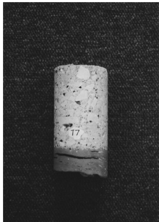
Fig. 6. Partial core showing large planar void in tile
